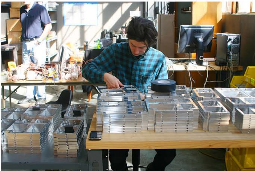
A Magico assembly technician wraps the aluminum parts where internal speaker wiring could contact the metal, thereby protecting the wires from potential tears.
