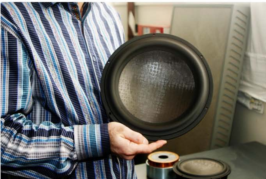
The massive 5" voice coil seen on this Magico driver is a sight to behold.
