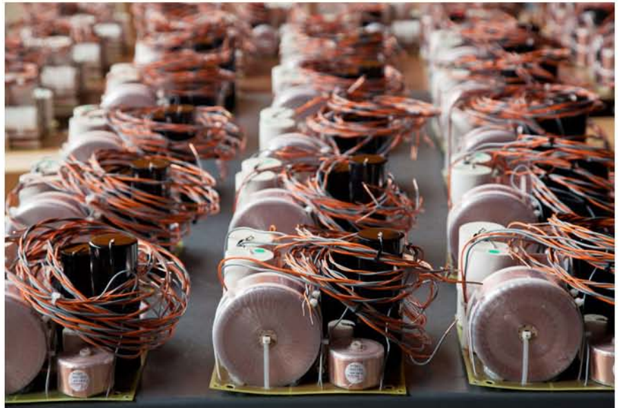
Crossovers consist of parts from Mundorf, a company located in Germany.
