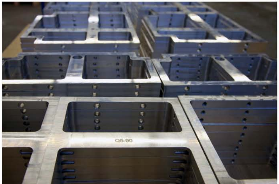
Q-series enclosures await driver insertion and final assembly.
