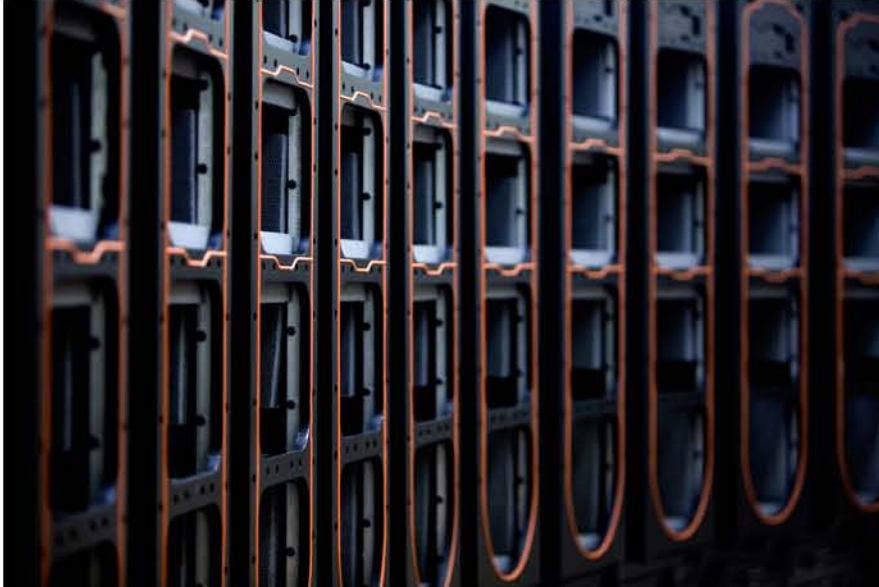
Q-series enclosures await driver insertion and final assembly.
